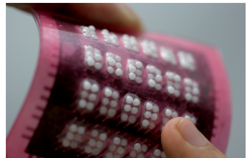
Figure 18. Flexible sheet scanner. Source: Prof. Takao Someya, University of Tokyo
