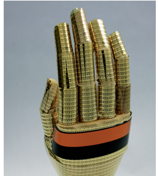
Figure 19. "Artificial skin" flexible integrated pressure and temperature sensors. Made by Prof. Takao Someya, University of Tokyo.
