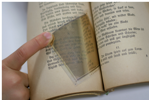
Figure 19. "Artificial skin" flexible integrated pressure and temperature sensors. Made by Prof. Takao Someya, University of Tokyo.
